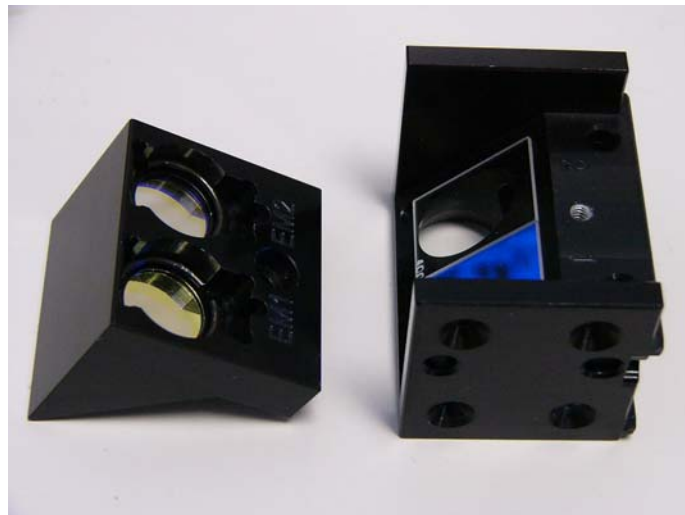
Figure 5: Filter cube with top removed
