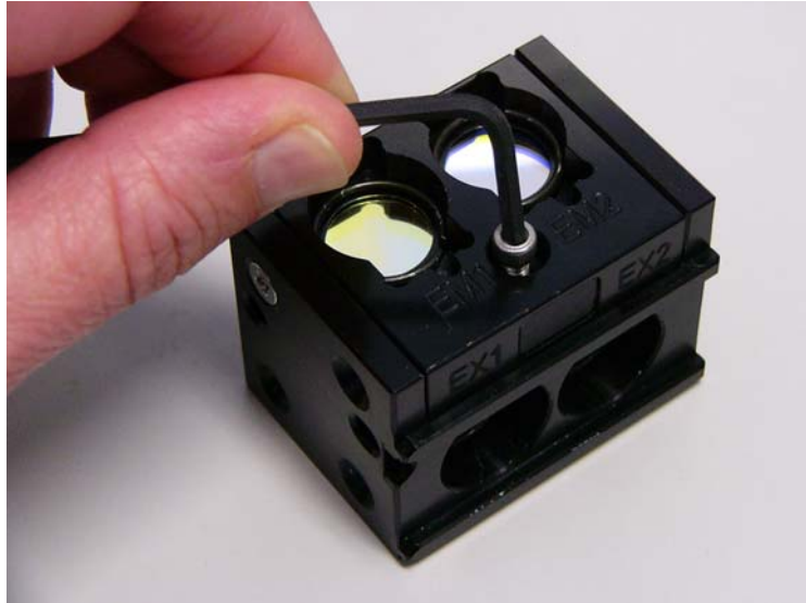
Figure 1: Remove the screw from between the EM1 and EM2 positions
