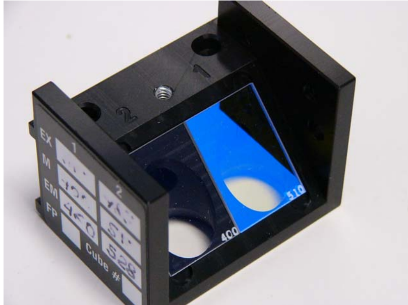
Figure 2: Mirrors positioned in the filter cube
